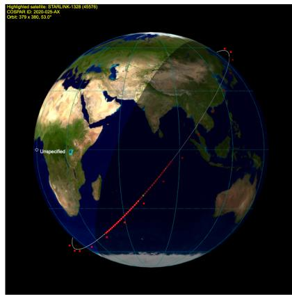
The satellites in the orbital plane in this image are still being deployed from their initial orbit at an altitude of around 380km. Notice, in particular, that there are a large number which are still closely spaced. These closely spaced satellites are responsible for the "chains" which have been observed by many astronomers.
